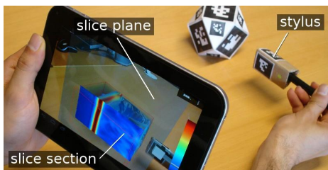
Figure 1: A virtual slice plane is attached to the stylus, which is manipulated with the fingers to slice through the dataset.
